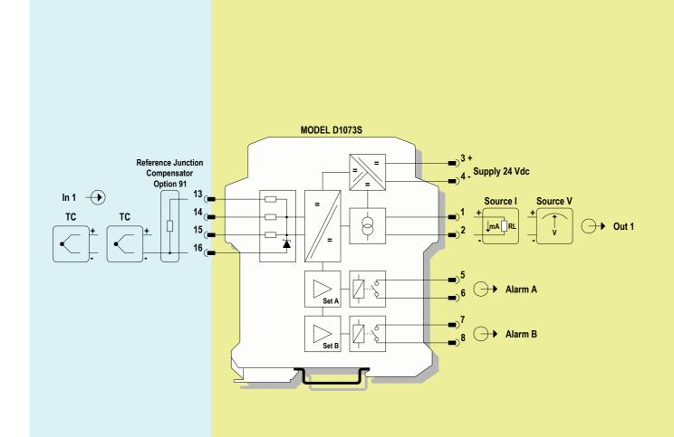
For SIL applications, alarm contacts must be used in series with equal configuration. Relay contact shown in de-energized position
