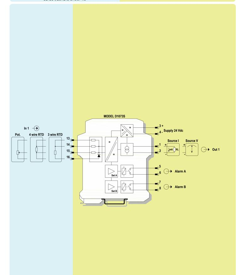
For SIL applications, alarm contacts must be used in series with equal configuration. Relay contact shown in de-energized position
